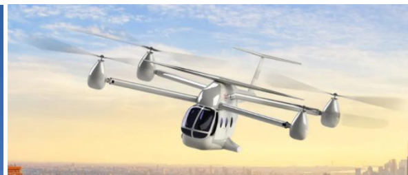
Figure 1 Rotor X eVTOL has 1600lbs lift and is slated for FRED testing.
